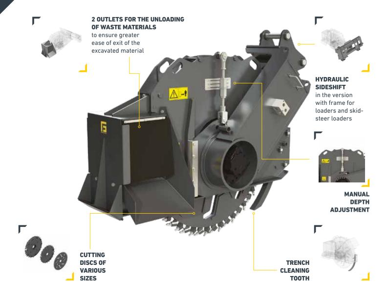
The wheel trencher is designed to carry out **excavations of different thickness and depth**, on hard and compact surfaces such as asphalt, concrete and rock, for the **installation of optical fibre** or other **cables** of any kind.
