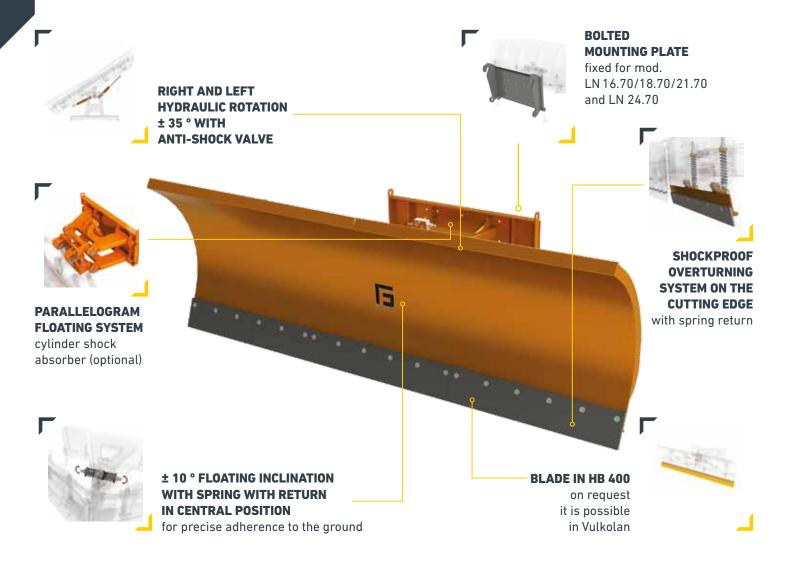
The snow plow blade is used to **clear snow** from yards, parking lots, courtyards, sports facilities and roads and is a **fundamental** piece of equipment for road traffic and **winter maintenance**.
