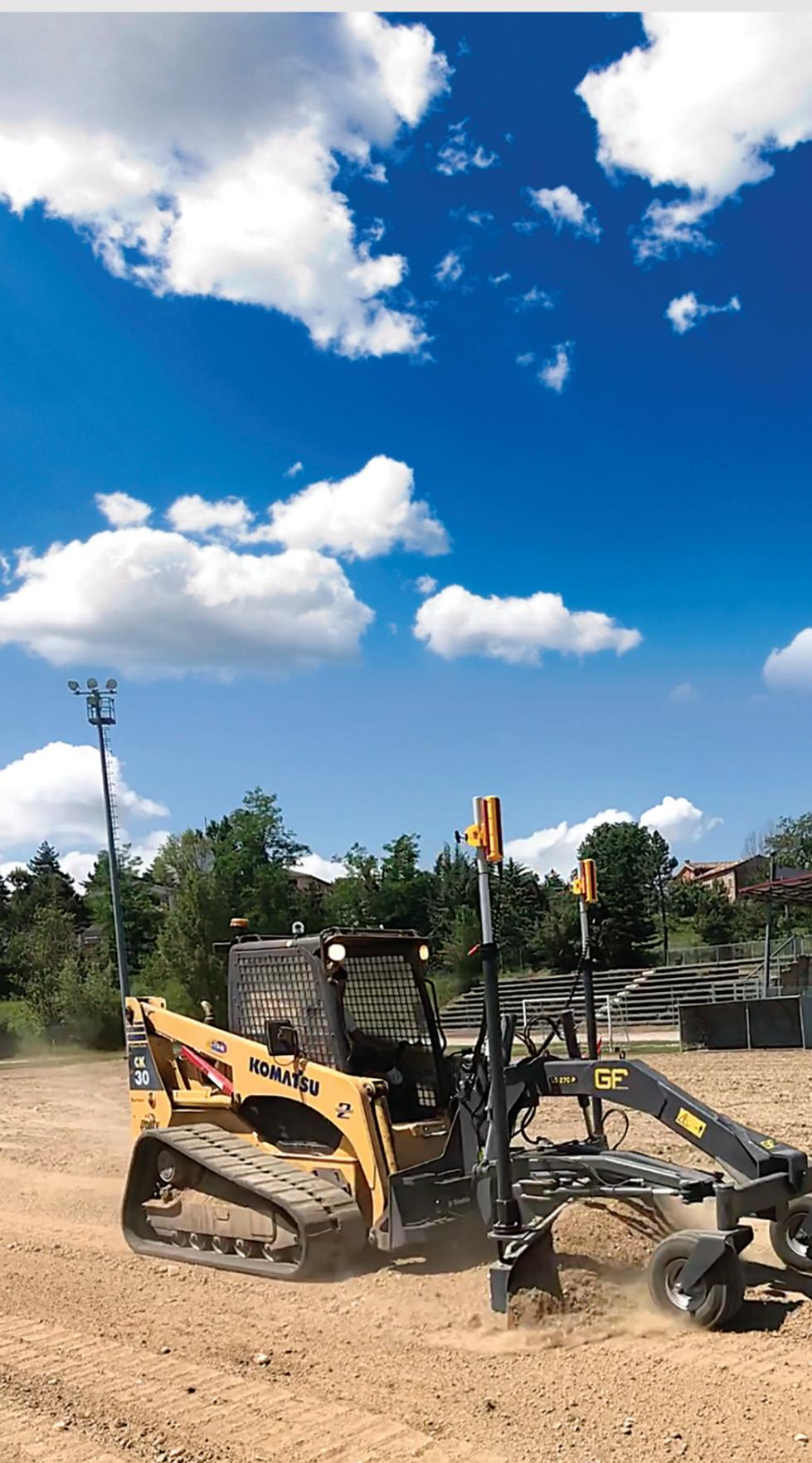
Trimble Earthworks GO! can be used by contractors involved in general construction, site preparation and utility work for grading flat and simple slopes. The system leverages laser technology to provide dynamic, real-time position information that allows the operator to grade or cut profiles quickly and accurately.
